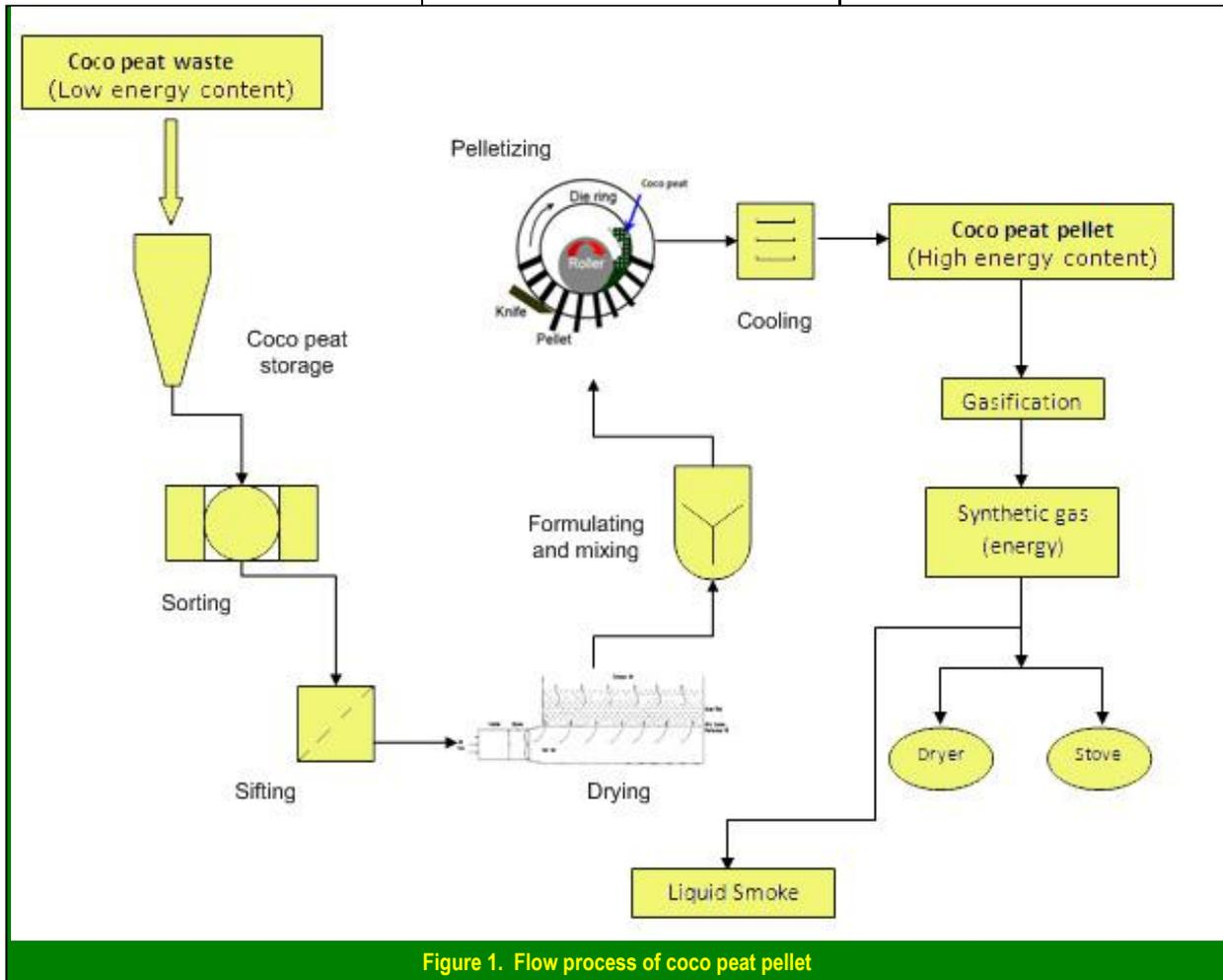
Figure 1. Flow process of coco peat pellet
