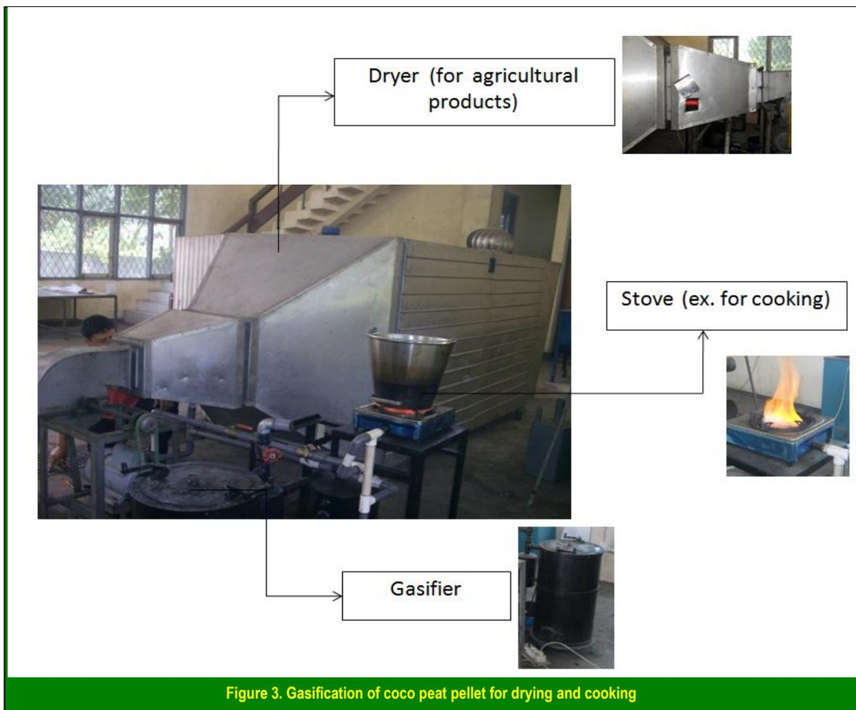
Figure 3. Gasification of coco peat pellet for drying and cooking
