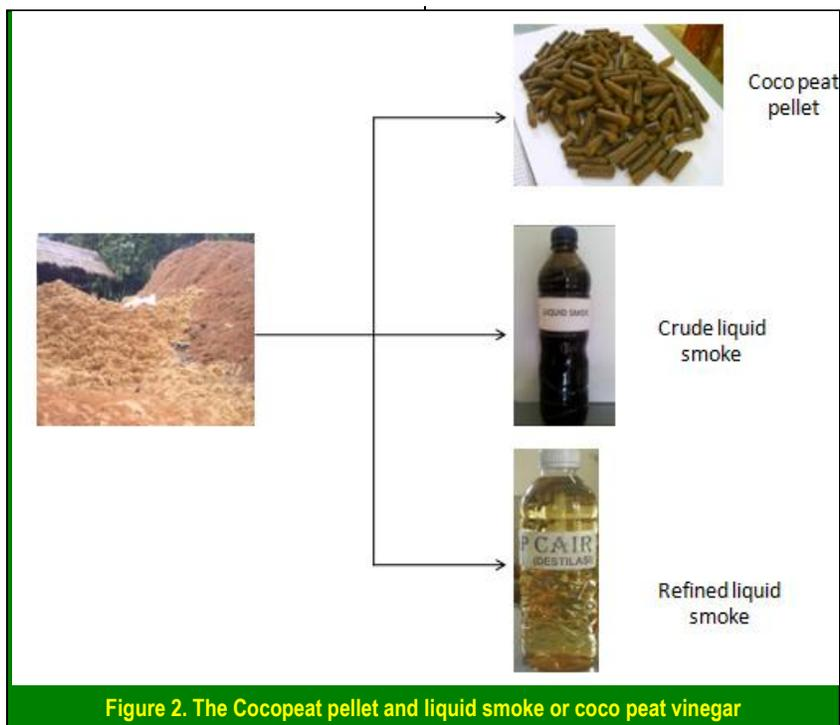
Figure 2. The Cocopeat pellet and liquid smoke or coco peat vinegar
